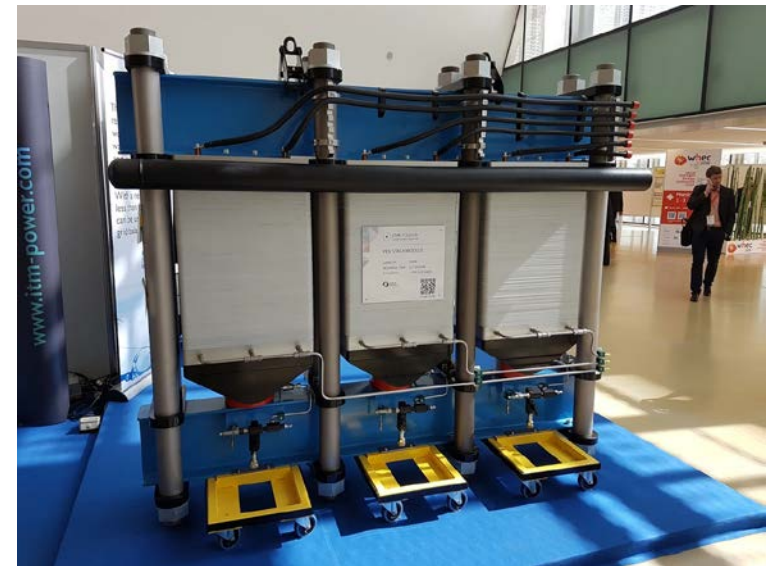
PEM electrolysis stack , 2 MW (ITM Power, WHEC 2016)
